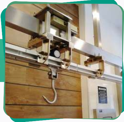
Industrial overhead weighing beams for meat handling.
