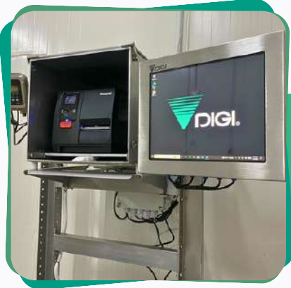
Industrial weighing station equipment - traceability.
